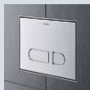
Flush-mounted installation The actuator plate can be fully integrated into the wall using an installation frame available separately. Only available for A1 in plastic white and plastic high-gloss chrome. Essential for initial structural construction. Suitable for dry-wall paneling with a minimum thickness of 25 mm.
