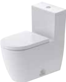
Set Toilet One-Piece Duravit Rimless® elongated with syphonic jet action, 305 mm/12” rough-in, with dual flush piston valve, top flush, vertical outlet. One-Piece Toilet incl. seat & cover w/ soft closure
