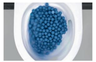
In trials with test balls, up to ten times more balls are flushed away than the standard testing (DIN EN 997-2018) requires.
